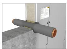
Incombustible pipes with unbroken (CS) synthetic rubber insulation, fire index number ≥ D-s3, d0)
