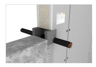
Cables / cable bundles in small penetration seal, circular and square (positive test findings, to be adopted in the ETA following the next revision)
